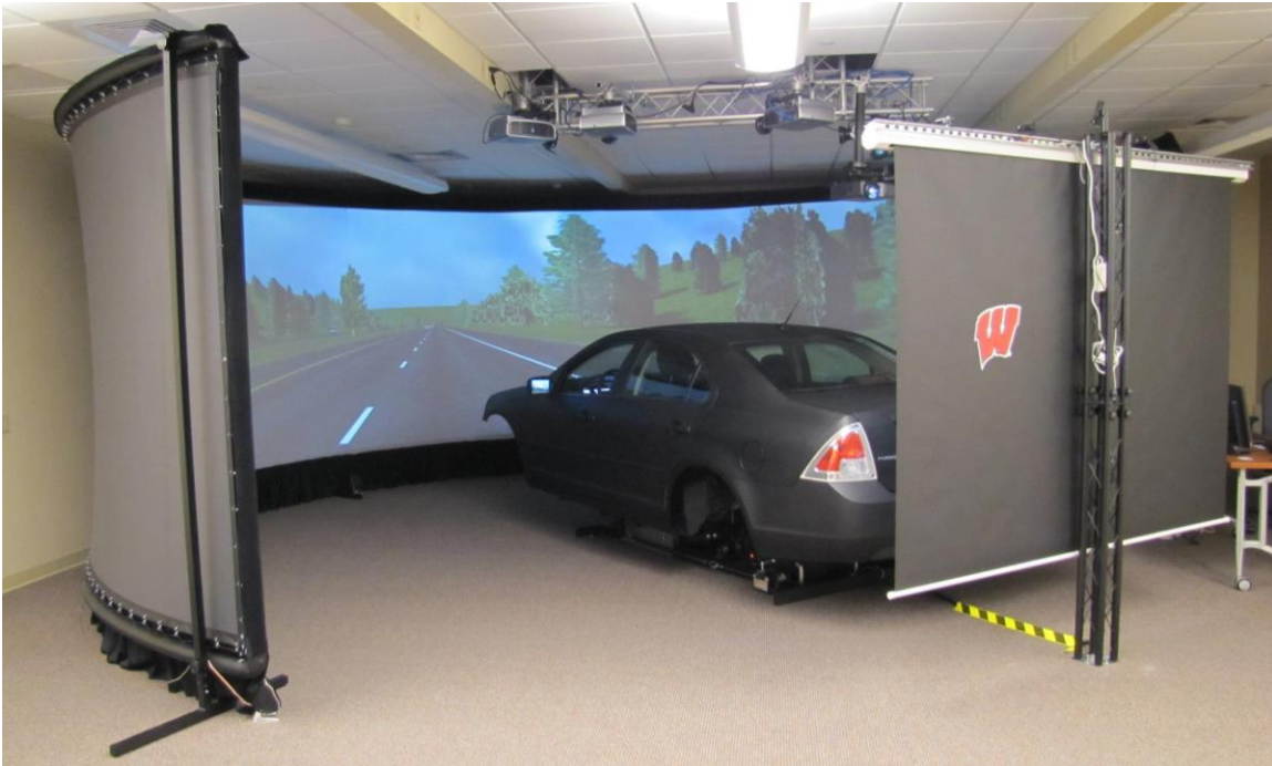
Figure 3.1 – Full-scale driving simulator at UW-Madison
